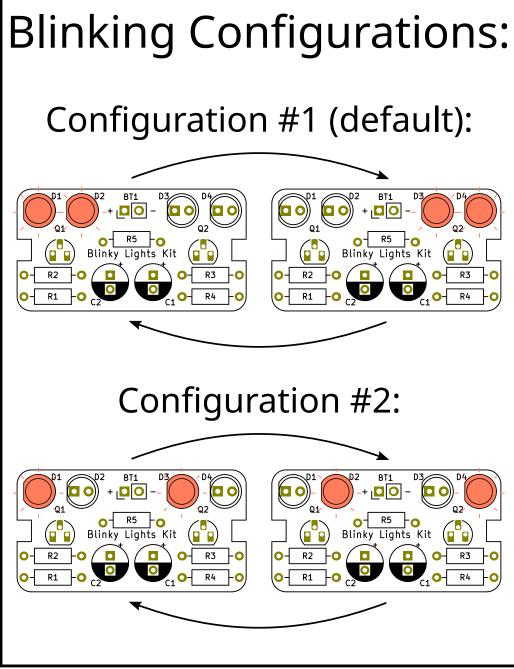
Note: All LEDs that are blinking at any one time (depending on which configuration is set) needs to be the same color when soldered on to the board.
